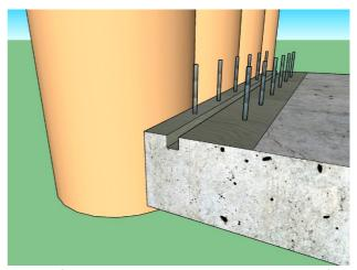
Using a natural bristle concrete brush coat the entire surface area of the cavity. Allow the application to dry for 1 to 2 hours.
